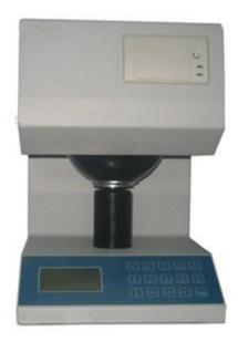
Brightness Meter is widely applied in paper and cardboard, pulp, cotton and fabric, plastic, ceramic and porcelain enamel, amylum, construction material, chemical industry, salt making and other testing department that need to test whiteness, yellowness, color and chromatism, as well as transparency, opacity, light scattering coefficient and light absorption coefficient of paper.
