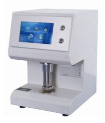
Bekk Smoothness tester is designed according to the Bekk type smoothness principle. Equipped with high-precision sensor and imported oil-free vacuum pump. Standards: ISO 5627
