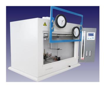
Burning behavior test for plastic, rubber and its products at the source of fire burning under the provisions in order to determine the material's fire rating. Standards: ASTM D635-1974, UL 94
