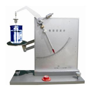
The meter is used to measure the density of rubber and similar material.
